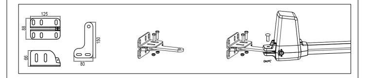
**Step 3:** Fix the operator on the rear bracket.
